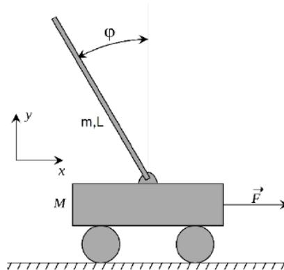
**Fig. 1.** Cart pendulum system. [1]
