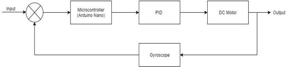
**Fig. 10.** Schematic diagram of electrical and electronic system.
