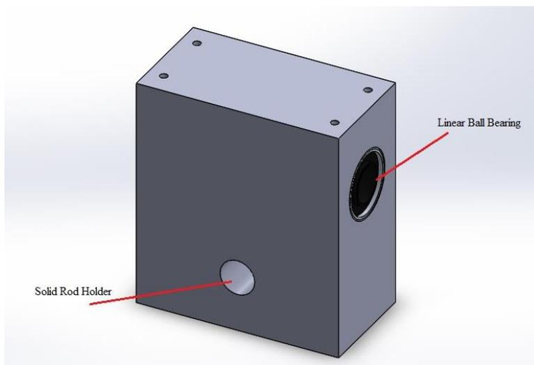
**Fig. 5.** Sliding mechanism.
