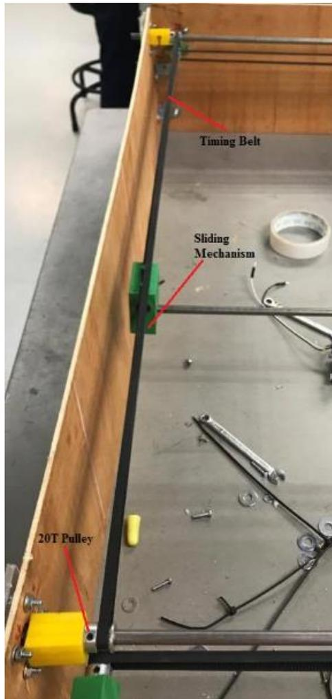
**Fig. 9.** Left end of stabiliser mechanism.
