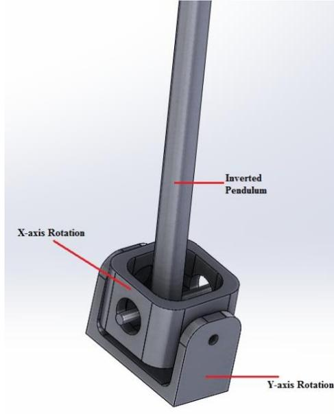
**Fig. 6.** Inverted pendulum holder.
