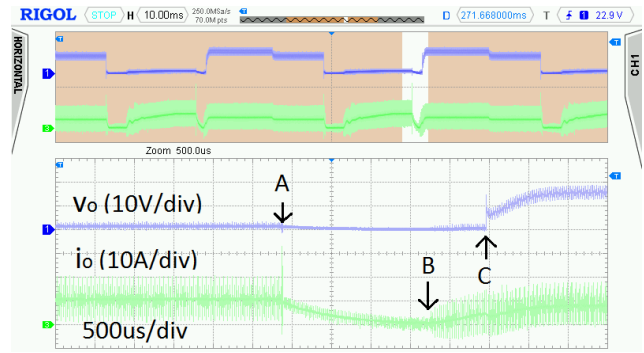
Fig. 17. Details of the waveforms in the transition from the short circuit phase to the arcing phase.
