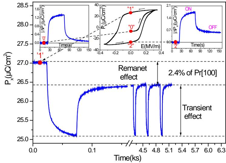
**Figure 2 | Photopolarization effect.** A sample initially in remnant state ‘1’, is illuminated by a UV (365 nm) diode. Within a few s, a change of polarization is established, with a fraction remaining after turning off the light (remanent effect). Subsequent illuminations only reveal the transient effect, with no more remanence. Insets show how the remanence in polarization depends on the FE state.
