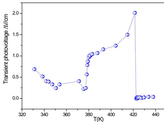
**Figure 5 | Temperature dependence of the photovoltaic effect.**
