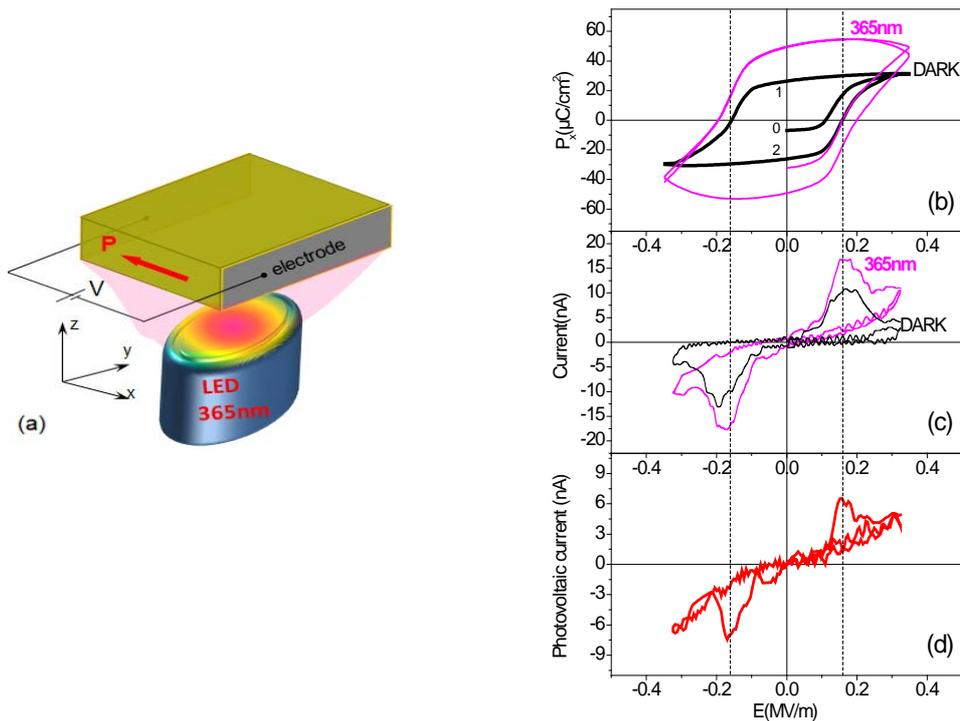
**Figure 1 | Photoferroelectric measurements details.** (a) Schematic of the experiment setup with respect to the crystalline axis. Ferroelectric polarization (b) and current (c) hysteresis loops in darkness and under 365nm irradiation. (c) Related photocurrent as a function of voltage.
