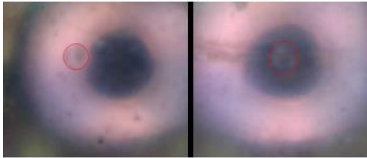
Fig. 6. Wear scar image from the optical microscope; Left: WS for sample 3 at 80 kg; Right: WS for sample 1 under 80 kg load.
