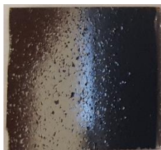
Fig. 2. Crack-like defects produced in \mu\text{-Si:H} thin films with post-annealing at 550°C for 1 h in air. Similar cracks appeared in samples of both 1 and 3 \mu\text{m} thickness which produced an abrupt drop in electrical conductivity.
