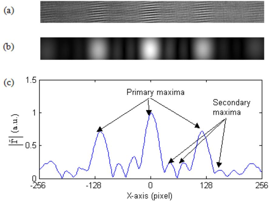
Figure 5. Interference of the spatial coherence function from four rectangular sources. (a) Interferograms obtained at  $Z = 0$ . (b) Reconstructed coherence function. (c) Curves of normalized  $|\tilde{\Gamma}(x, 0, 0)|$ .
