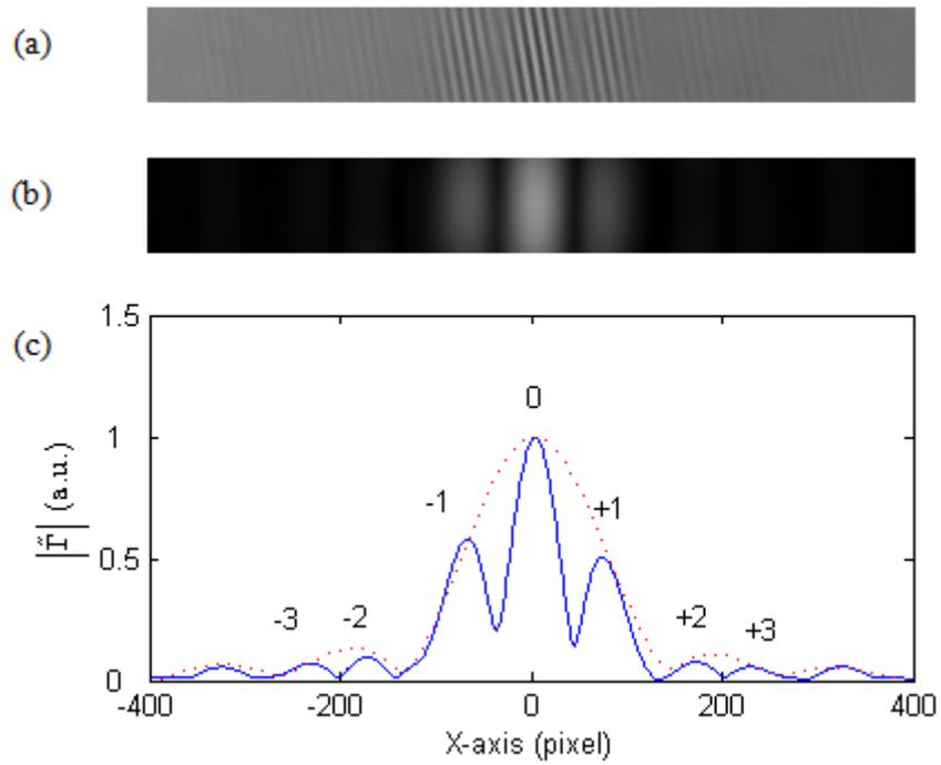
Figure 3. Coherence function from two rectangular sources. (a) Interferogram obtained at  $Z=0$ . (b) Reconstructed coherence function. (c) Curves of normalized  $|\tilde{\Gamma}(x,0,0)|$ , where the dotted line is the coherence function from a single rectangular source and the solid line is the coherence function from two rectangular sources.
