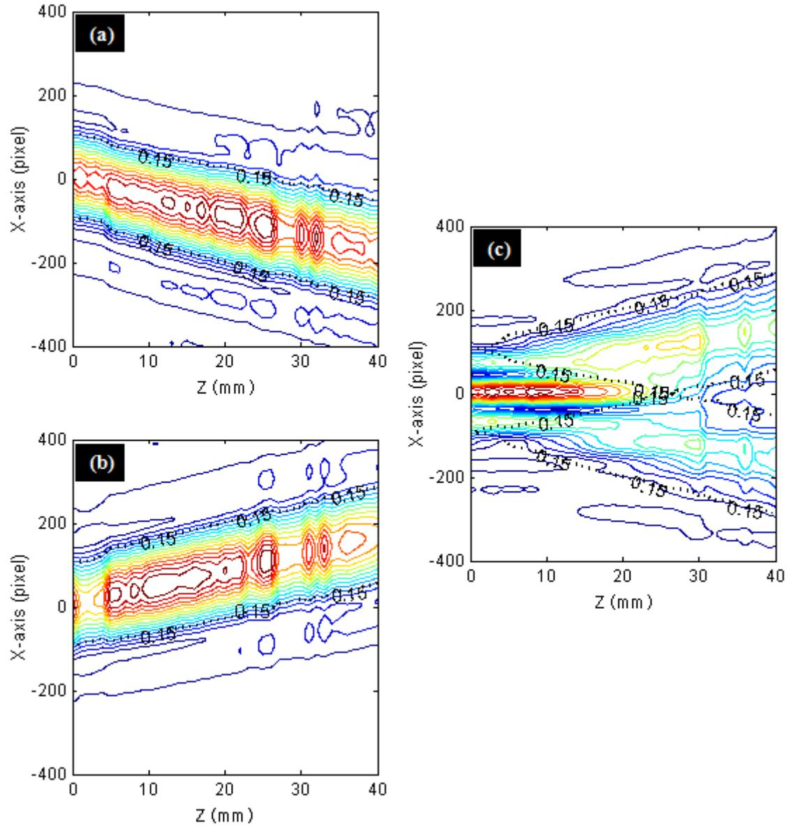
Figure 6. (a) Contour map of the coherence function originates from source  $I_1$ . (b) contour map of the coherence function originates from source  $I_2$ . (c) contour map of the interference of coherence functions from the two sources. Dotted contour lines with value of 0.15.
