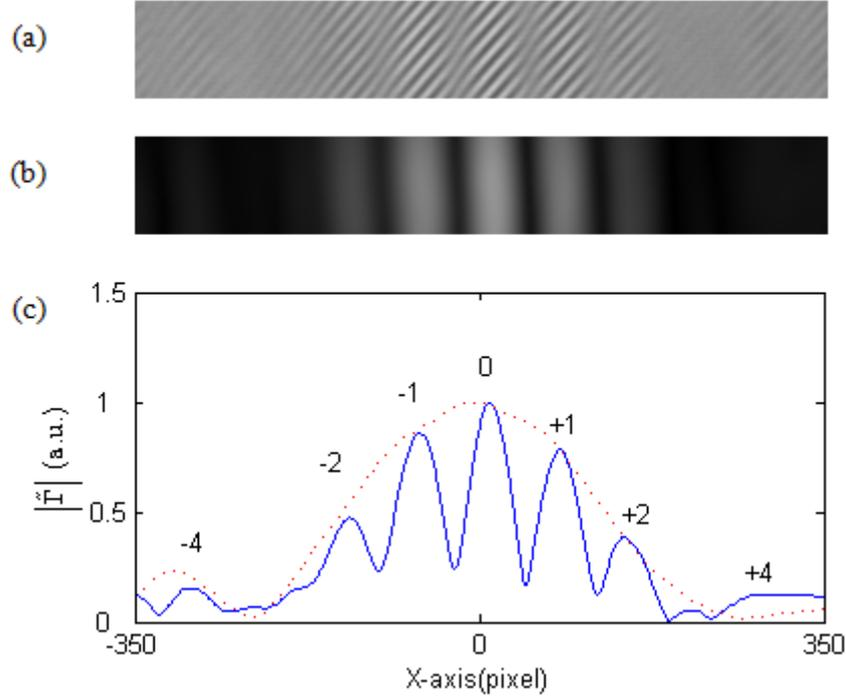
Figure 4. Coherence function from two rectangular sources, with spacing ratio of hole pitch and hole size is 3:1. (a) Interferogram obtained at  $Z=0$ . (b) Reconstructed coherence function. (c) Curves of normalized  $|\tilde{\Gamma}(x,0,0)|$ , where the dotted line is the coherence function from a single rectangular source and the solid line is the coherence function from two rectangular sources. Missing orders occur at  $\pm 3$ .
