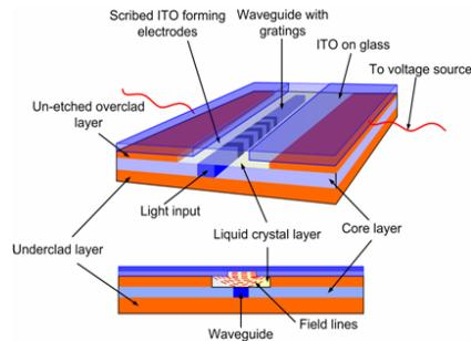
**FIGURE 3.** Configuration of liquid crystal tuned grating device.
