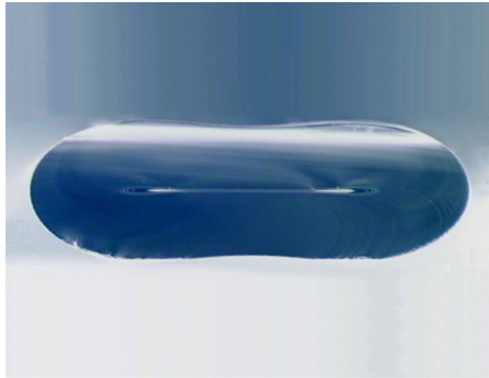
FIGURE 5. Showing a cross-section of a flat-fibre UV writing substrate.
