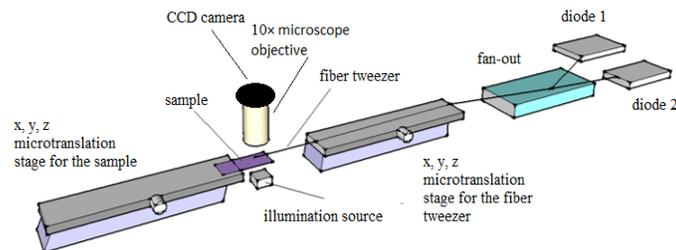
Fig. 5. Experimental set-up for using the machined MCF-based optical tweezer.
