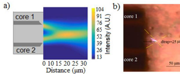
Fig. 4. Beam propagation for the two machined, diagonally opposite cores as seen from the cross-section of the multicore fiber. a) Matlab simulation of the beam propagation from the two cores. The overlapping 'trapping' area can be clearly seen when the two weakly diverging beams cross. b) Optical image of yeast cell. Core 1 and core 2 are annotated on the image and the laser light scattered by the yeast cells indicates the beam propagation angle.
