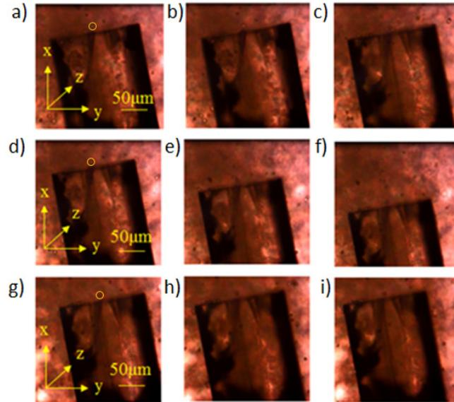
Fig. 6. Trapped yeast cell using 4.9 mW and 17.2 mW optical power from core 1 and 2 respectively. a)-c) Movement in z axis d)-f) movement in x axis and g)-i) movement in y axis. The trapped particle is shown inside the yellow circle.
