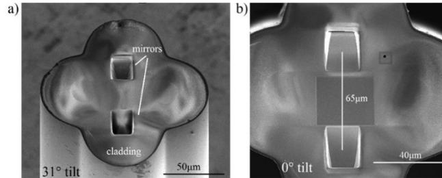
Fig. 3. a), b) Scanning electron microscope (SEM) micrographs of fiber surface after mirror fabrication on two diagonally opposite cores, when the fiber end-face is tilted in  $31^\circ$  and  $0^\circ$  with respect to the SEM, respectively. b) A dark square in the centre of the fiber can be seen and it is due to the gold layer removal using the FIB, in order to eliminate the heating effect through the trapping experiment.
