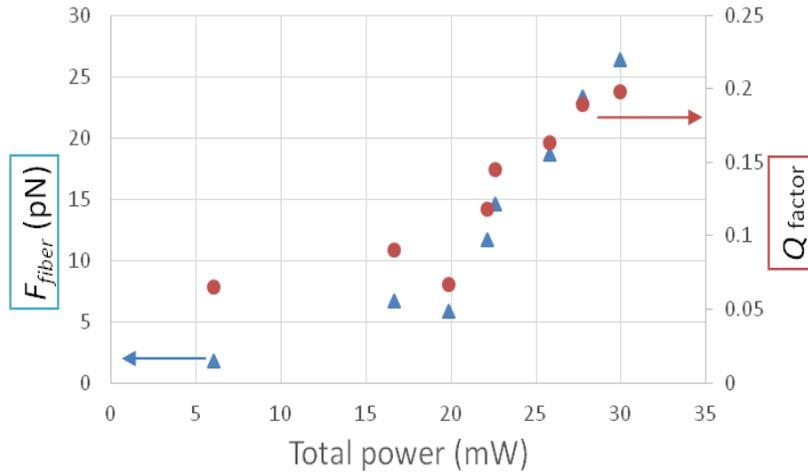
Fig. 7. Blue triangles: Experimental values of the fiber force ( $F_{fiber}$ ) which were calculated by equating the trapping force of the OT ( $F_{trap}$ ) that broke the fiber trap. Orange circles: The efficiency factor  $Q$  for different total powers of the tweezing probe.
