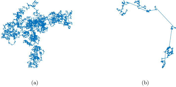
FIG. 2. Illustration of trajectories of a Brownian motion (2a) and a Lévy walk (2b) in two dimensions. The Brownian motion trajectory was obtained using a running probability function \psi = e^{-\tau} and for the Lévy walk \psi = \left(\frac{1}{1+\tau}\right)^\alpha for \alpha = 1.5 . The angle \theta for the new direction is chosen from a uniform distribution in both cases.
