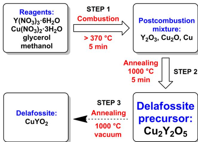
**Fig. 1.** General synthetic procedure for obtaining  $\text{Cu}_2\text{Y}_2\text{O}_5$ .
