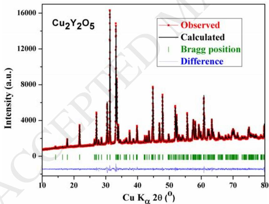
**Fig. 4.** Profile matching to the XRD pattern of  $\text{Cu}_2\text{Y}_2\text{O}_5$  synthesized at  $1000\text{ }^\circ\text{C}/5\text{ min}$ ; the observed (red points), calculated (black solid line), Bragg positions (green bars) and
