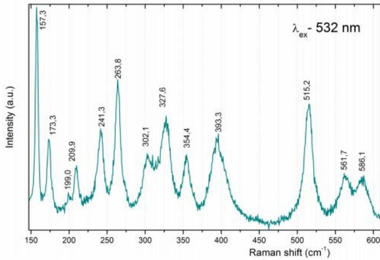
**Fig. 7.** Fourier transform Raman spectrum of  $\text{Cu}_2\text{Y}_2\text{O}_5$  obtained at  $1000\text{ }^\circ\text{C}/5\text{ min}$ .
