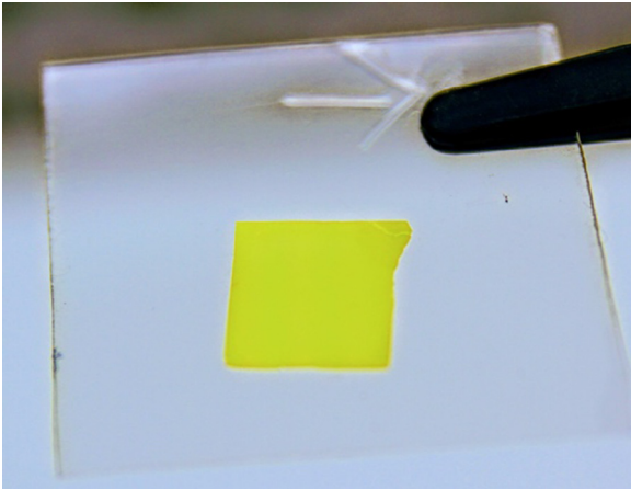
Fig. 2. Image of 5 \times 5 mm ZnSe ELO layers transferred onto glass plates from (2 1 1) B substrate.
