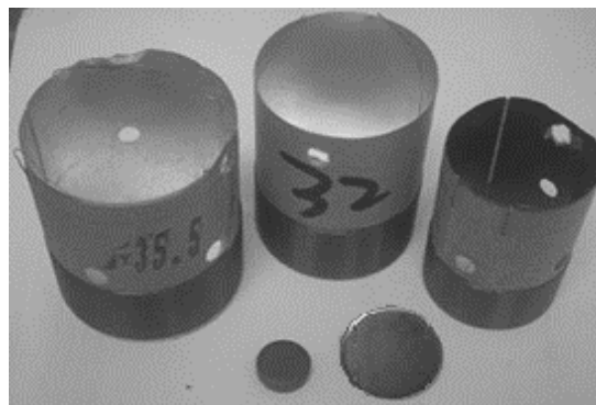
Figure 2: Voice coils of various diameter and two different permanent magnets
