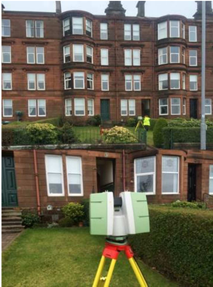
Figure 3.3D laser scan of Façade
