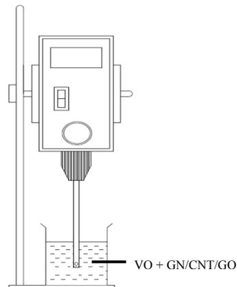
**Figure 1.** Schematic set-up of high speed homogenizer.
