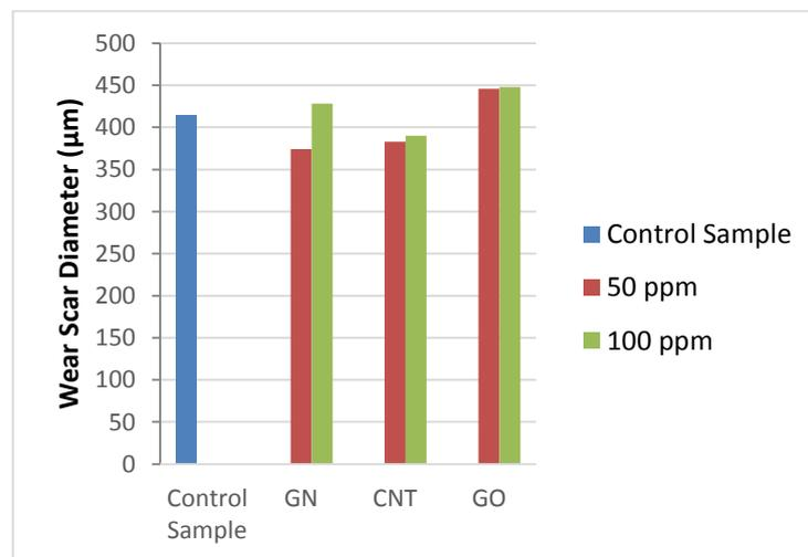
**Figure. 6.** Wear scar diameter against 50ppm and 100ppm GN, CNT and GO
