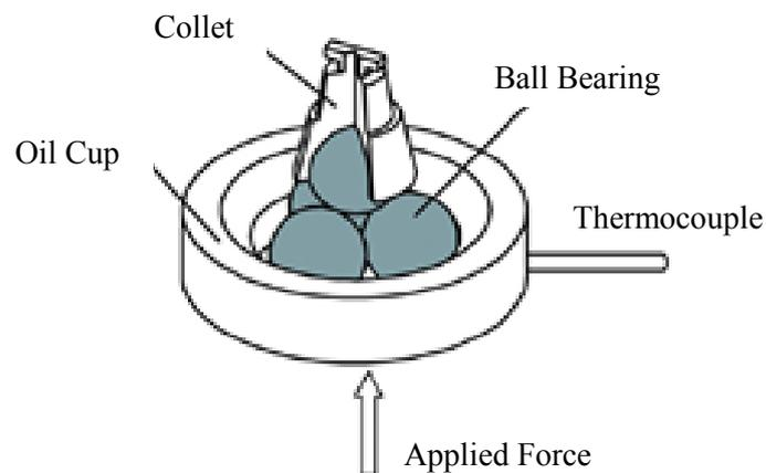
**Figure 2.** Schematic diagram of four ball setup in experiment [10]
