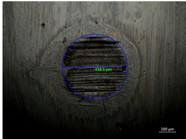
**Figure. 3.** Wear scar diameter measured on one of the sample ball
