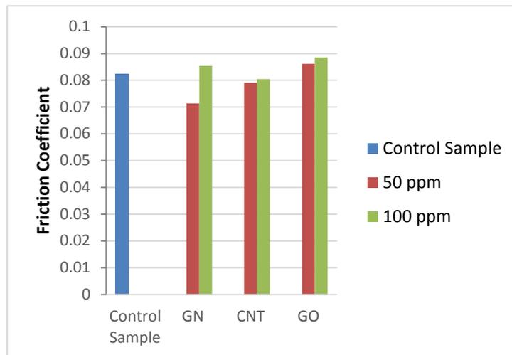
**Figure. 5.** Friction coefficient against 50ppm and 100ppm GN, CNT, and GO
