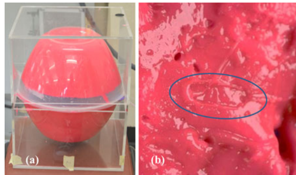
Fig. 6. (a) Entire phantom setup. (b) Indentation of capsule in phantom.
