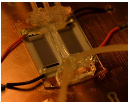
Figure 2. Photograph of surface acoustic wave device with a bonded PDMS microfluidic channel on a printed circuit board.
