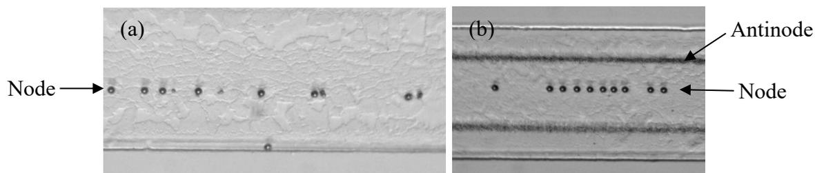
Figure 3. 10  $\mu\text{m}$  commercialised and 4.6  $\mu\text{m}$  custom made micro-particles aligned (a) at the nodal position of the surface acoustic standing wave, (b) at the node and antinode positions of the surface acoustic standing wave, respectively.
