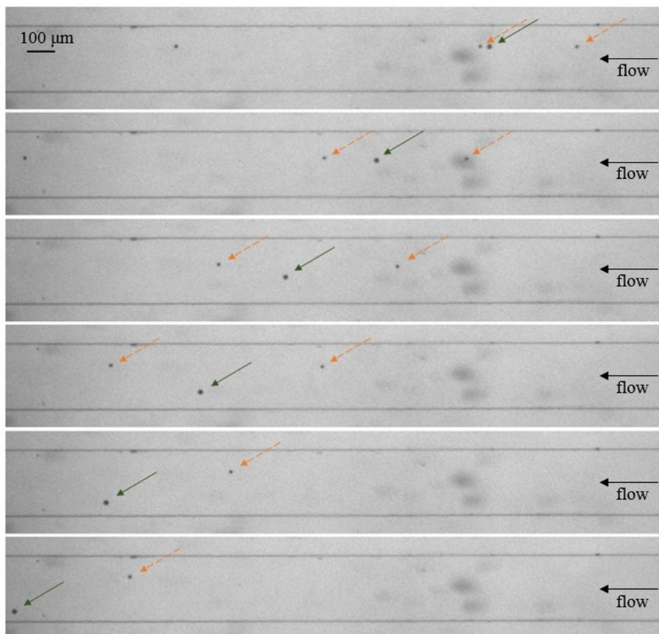
Figure 4. Images showing the separation process for 0.7 s ramping time. The 15 (green, solid) and 10 (orange, broken)  $\mu\text{m}$  particles enter from the top right and the larger one is shifted to the bottom. The flow is from the right to the left. The frames are taken every 0.3 s.
