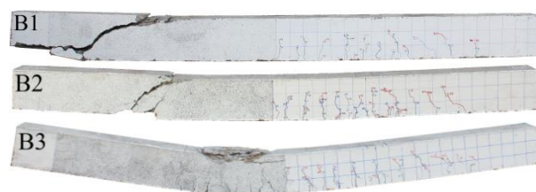
Figure 5. Crack Patterns after Failure
