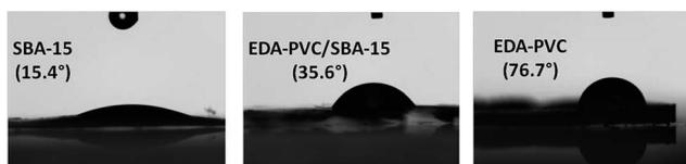
Fig. 9 Images from the contact angle measurement experiment on SBA-15, EDA-PVC/SBA-15 (4%) and unsupported EDA-PVC polymer.
