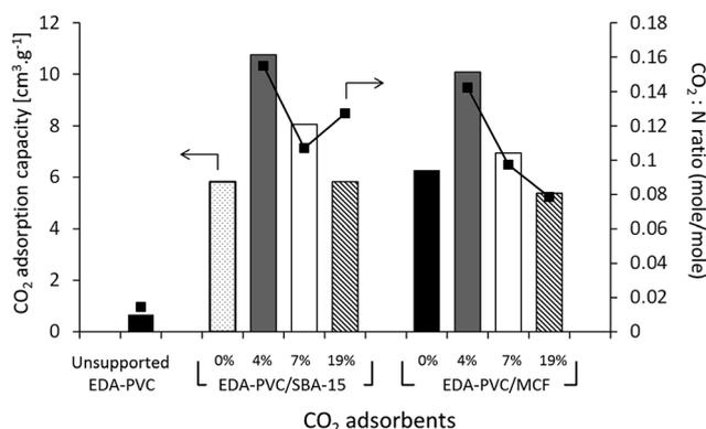
Fig. 6 CO<sub>2</sub> adsorption capacity at 25 °C measured by gravimetric method (left scale) and CO<sub>2</sub>:N ratio (right scale) for EDA–PVC/mesoporous silica samples depending on the amount of APVC. The CO<sub>2</sub>:N ratio is calculated from the CO<sub>2</sub> adsorption capacity while the nitrogen content was calculated from CHN analysis.
