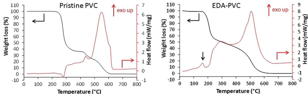
Fig. 2 TGA (black, left scale) and DSC (red, right scale) for unmodified PVC and EDA-PVC. The exothermic transition at around 160 °C (indicated with a black arrow) appeared only with cross-linkable aminated PVC samples.
