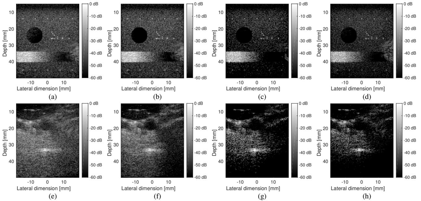
Fig. 2: Image of the numerical phantom reconstructed with (a) DAS - 1 PW insonification, (b) DAS - 5 PW insonifications, (c) USSR-SA - 1 PW insonification, (c) USSR -  $\ell_p$  - 1 PW insonification; Image of the *in-vivo* carotid reconstructed with (e) DAS - 1 PW insonification, (f) DAS - 5 PW insonifications, (g) USSR-SA - 1 PW insonification, (h) USSR- $\ell_p$  - 1 PW insonification.
