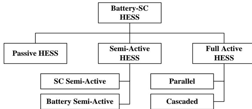
*Fig. 1. Classification of the Battery-SC HESS Connection Topologies [49][50]*
