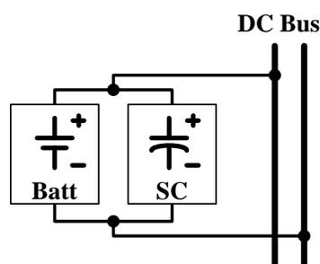
*Fig. 2. Passive HESS Topology*
