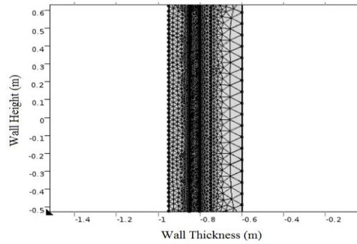
Fig. 6: Mesh of the CFD model of the dynamic wall construction
