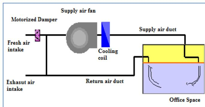
Fig 8. Schematic of the proposed cooling system
