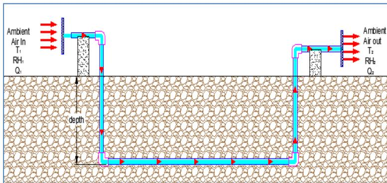
Fig. 1: Schematic drawing of the integrated EATS system
