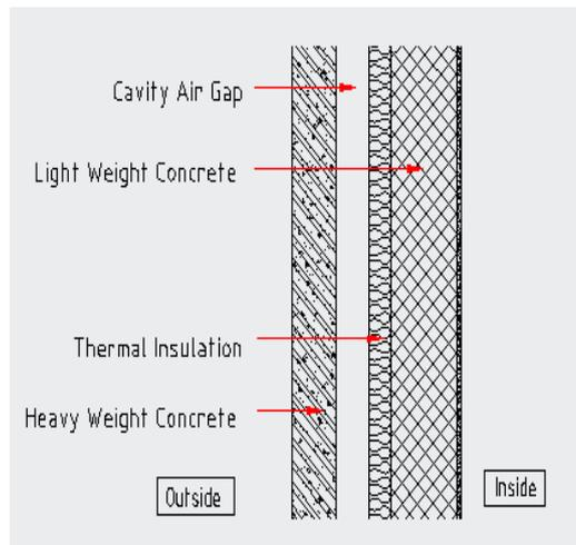
Fig.3: Cross section of the external wall construction
