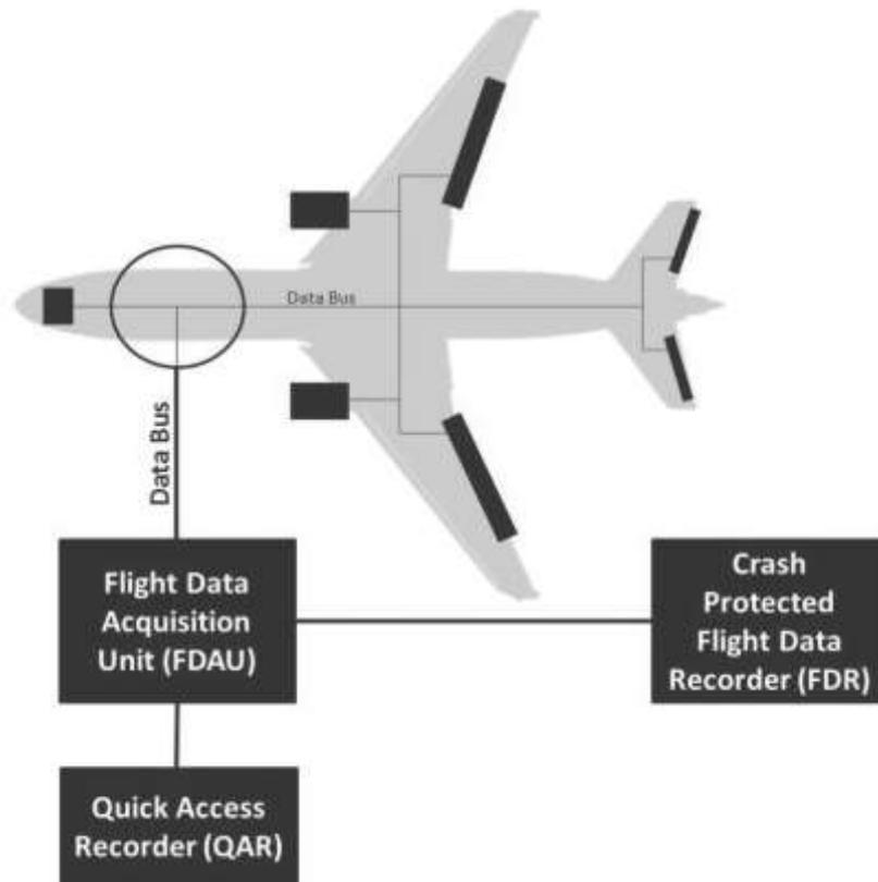
**Figure 3 – High level aviation data recording architecture**
