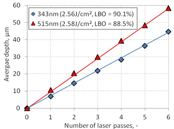
Figure 2. Average ablation depth at different number of laser passes. Results obtained at  $\lambda = 343$  and 515nm, for similar values of the average laser fluence and the laser beam overlap (LBO).
