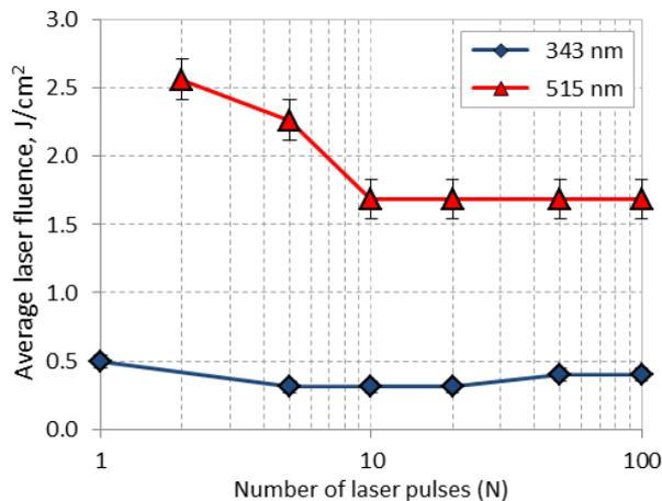
Figure 1. Surface damage threshold of Borofloat®33 glass determined at  $\lambda = 343$  and 515 nm.
