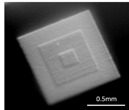
Figure 3. Structure machined in Borofloat®33 glass with a picosecond laser at  $\lambda = 515$  nm,  $F = 3.55\text{J}/\text{cm}^2$ , and  $\text{LBO} = 88.5\%$ .
