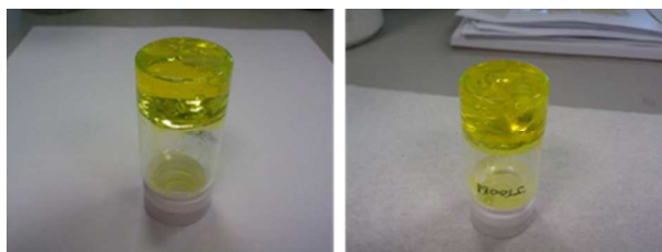
Figure 1. Inverted reaction vials showing Gel (3%) (left) and Gel (5%) (right) as insoluble gels swollen in chloroform.
