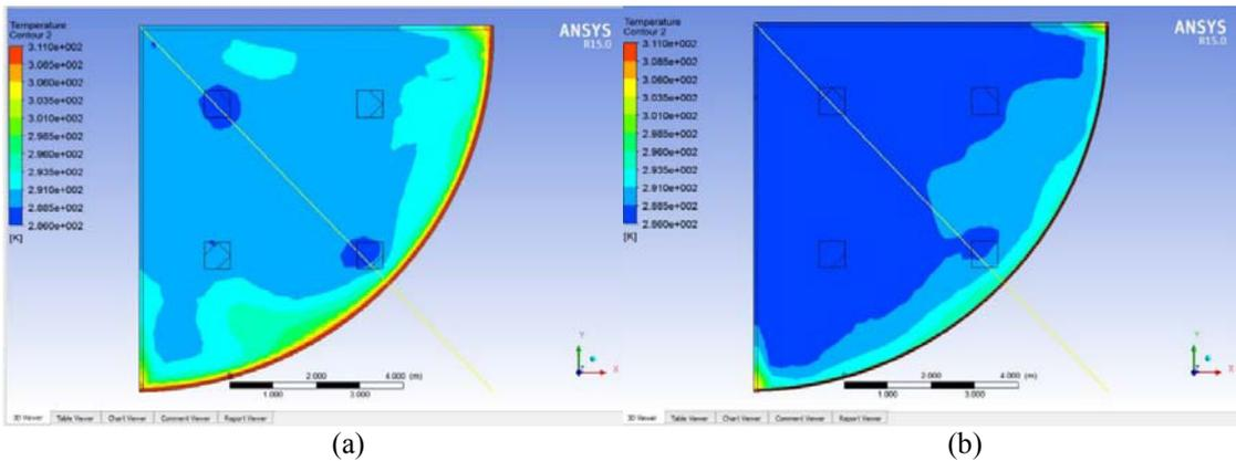
Figure 4: (a) Temperature Distribution without PCWW; (b) Figure 4: Temperature Distribution with PCWW
