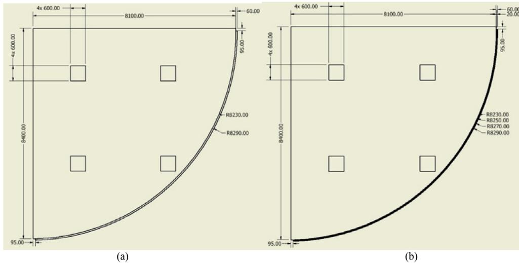
Figure 3: View from the top showing the air-conditioning inlet and the thickness of the (a) glass without PCWW and (b) glass with PCWW.
