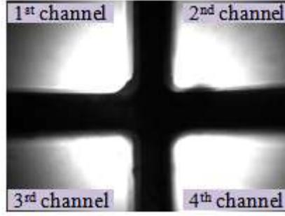
Figure 4. Image array on the CCD sensor: the 1st channel corresponds to  $\Gamma_{xx}(\tau)$ ; the 2nd channel corresponds to  $\Gamma_{yy}(\tau)$ ; the 3rd channel corresponds to  $\Gamma_{yx}(\tau)$ ; the 4th channel corresponds to  $\mathcal{I}(\tau)$ .
