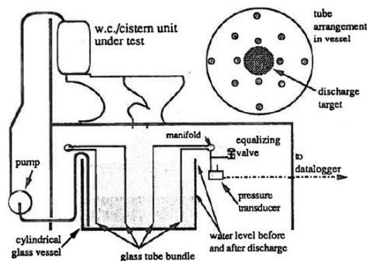
**Figure 1 Schematic diagram of the device used to measure the flush characteristics of the tipping tank. It averages the air pressure increase in 12 glass tubes submerged in a tank of known dimensions (Swaffield, J. A. 1993)**
