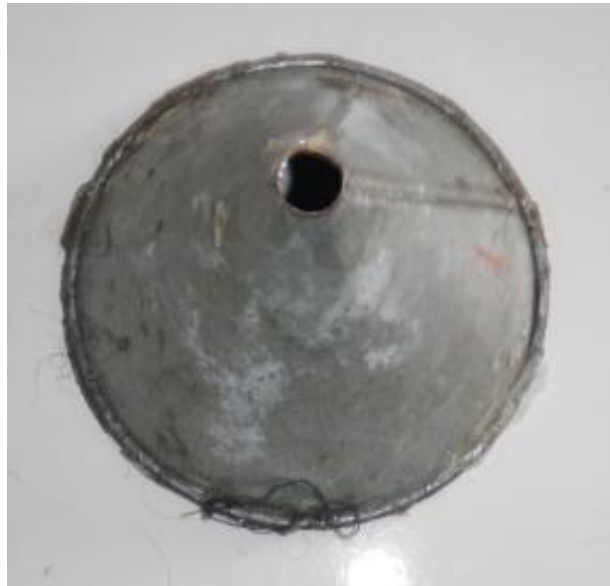
Fig. 2. Aluminum conical mandrel
