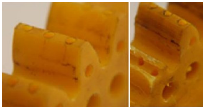
Figure 2. The damage in newly designed gears (Hayrettin, 2009)
