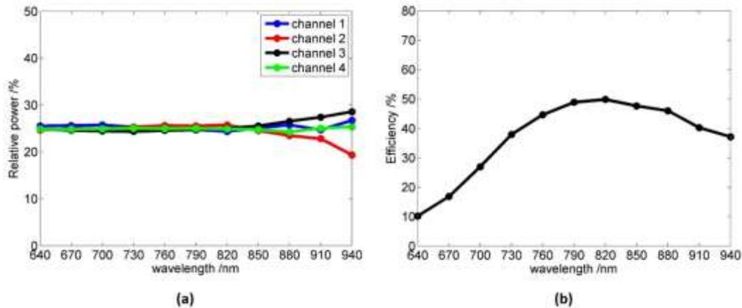
**Figure S1.** Relative power of each channel and total conversion efficiency. (a) Measured relative power in each channel of the metasurface. (b) Experimentally obtained conversion efficiency of the metasurface. The conversion efficiency is defined as the total power of four output beams divided by the power of incident light.
