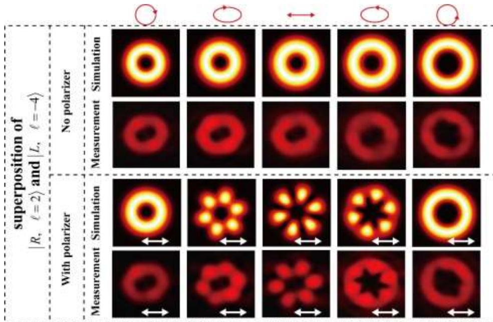
**Figure S2.** Simulated and measured intensity profiles of hybrid-OAM superposition states  $|R, \ell=2\rangle$  and  $|L, \ell=-4\rangle$ . The polarization states of incident light and the direction of the polarizer's transmission axis in front of the CCD camera are respectively denoted by the red symbols and the white double-headed arrows.
