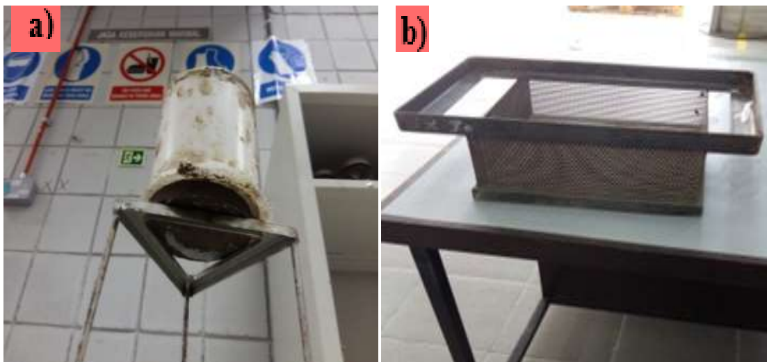
253 Fig. 5: Permeability setup for a) Prototypes samples b) Standard tiles
