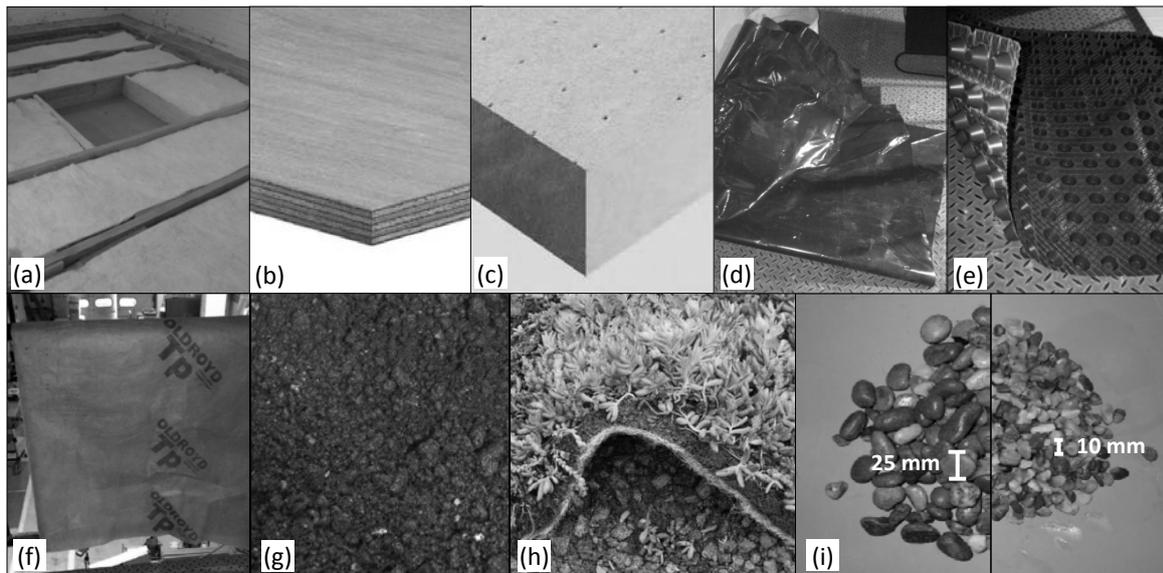
**Fig. 3.** Materials used for the green roof samples. (a) Timber joist floor with mineral wool insulation (open on top for illustration purposes); (b) Plywood; (c) Insulation board; (d) Waterproof membrane; (e) Drainage membrane; (f) Filter fleece; (g) Top soil; (h) Sedum mat; (i) Pebbles (*left*) and gravel (*right*).
