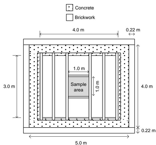
**Fig. 2.** Plan showing the separating floor and the 1 m<sup>2</sup> sample area used for green roof samples (not to scale).
