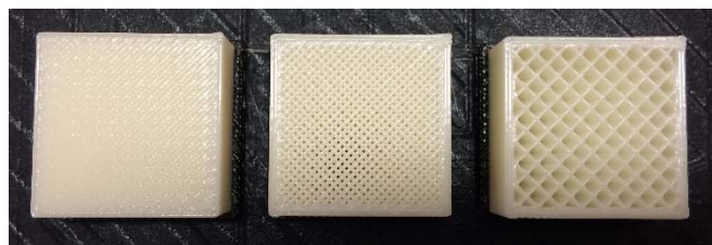
Fig. 1. Left to right, respectively: Internal structure of solid, high density, and low density FDM cubes.
