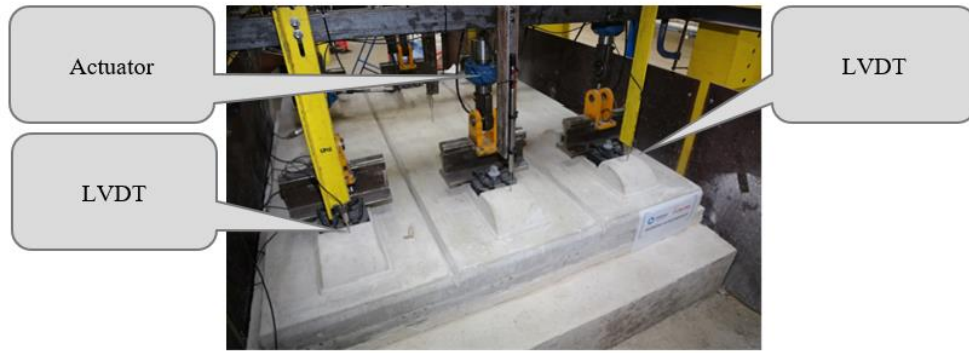
Figure 2 – GRAFT II test facility - Actuators and LVDTs
