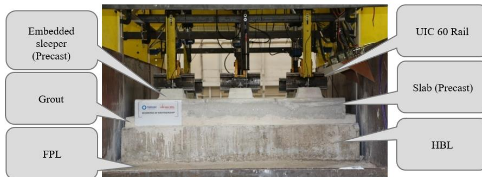
Figure 1 – GRAFT II test facility– Slab track system
