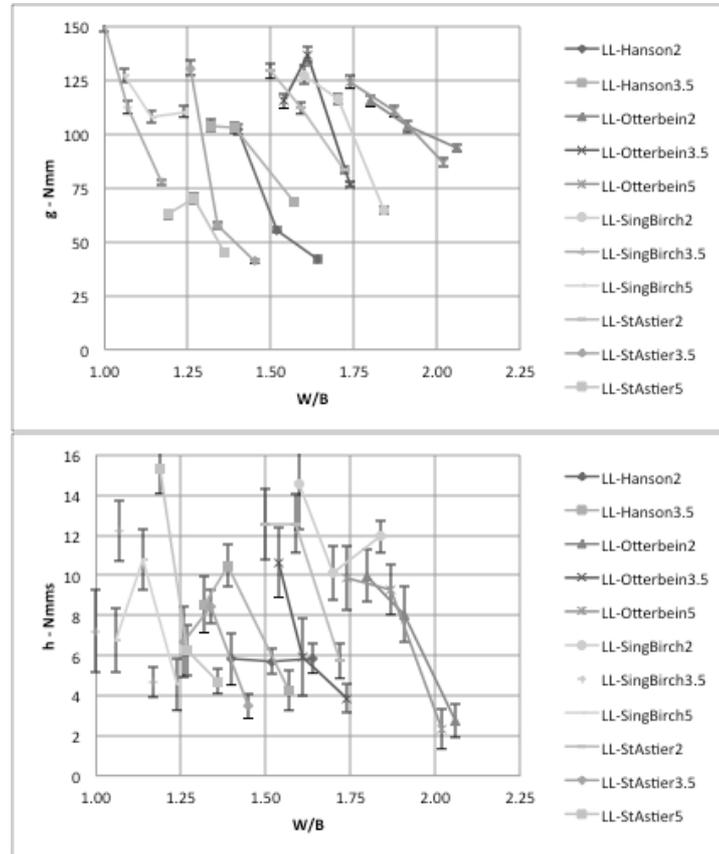
**Fig. 5** Effect of water content on  $g$  (above) and  $h$  (below) of Loanleven mortars
