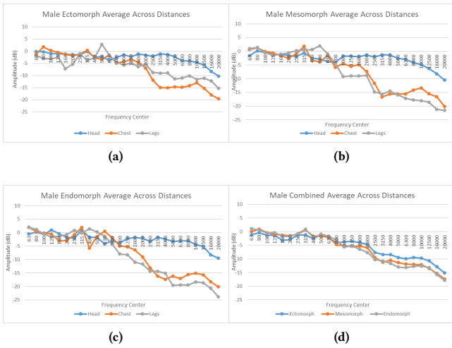
Figure 7: Averaged values across all distance measurements for male body types at head, chest and legs. Images (a),(b) and (c) show average values across distance for each microphone in the array for the three male measured body types (Ectomorph, Mesomorph and Endomorph). Image (d) illustrates the combined average of the microphones for each body type.
