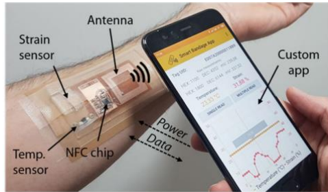
Fig. 12. NFC-based smart bandage attached to the arm for wireless strain and temperature monitoring using a custom smartphone app. (CC-BY).
