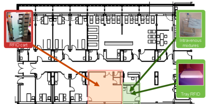
Fig. 26. UHF RFID for the traceability of intravenous mixtures. Reproduced by permission from open access article from MDPI Sensors (CC-BY).
