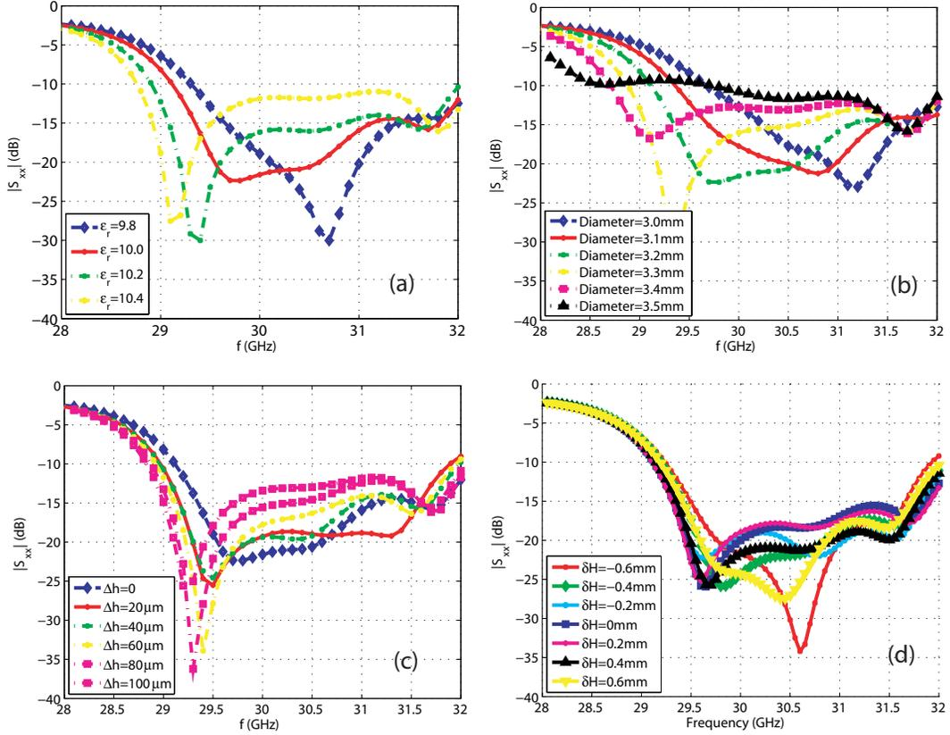
Fig. 5. Effect of fabrication parameters on the port reflection coefficient, (a) effect of  $\epsilon_r$  variations (b) effect of glue residue diameter, (c) effect of glue height and (d) effect of horizontal shift placement.
