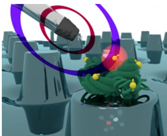
Figure 1 An artist's rendition of NanoMRI for molecular structure. © 2017, Philipp Scheiger. The figure depicts an array of diamond nanopillars, each hosting an NV center. The molecule of interest is placed on the diamond surface, and a magnetic field gradient enables an improved nanoMRI spatial resolution.
