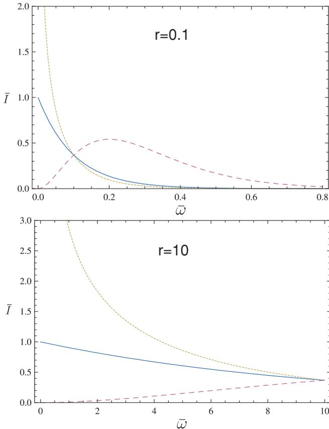
FIG. 1. (Color online) Spectral distributions  $\bar{I} = I/(g^2 k_B T)$  for the Ohmic (solid), super-Ohmic (dashed), and sub-Ohmic (dotted line) high- $T$  reservoirs, vs  $\bar{\omega} = \omega/\omega_0$ . In the upper figure we plot the off-resonant  $r = 0.1$  case, while the lower figure shows the  $r = 10$  case. For each spectral curve the location of the cutoff frequency is given by  $\bar{\omega}_c = \omega_c/\omega_0 = r$ . The location of the system oscillator frequency is always 1.
