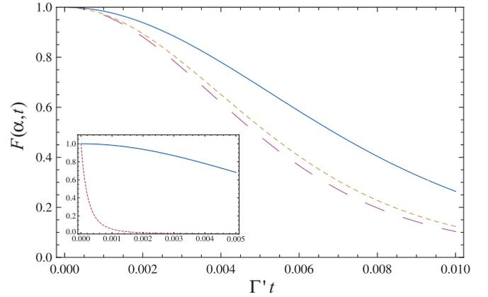
FIG. 3. (Color online) Fringe visibility for  $r = \omega_c/\omega_0 = 10$  for the Ohmic (solid), super-Ohmic (dashed) and sub-Ohmic (dotted line) reservoirs. The inset shows the comparison between non-Markovian (dotted line) and Markovian (solid line) fringe visibility for the Ohmic reservoir. Plots are given in unitless time  $\Gamma't = 2g^2\omega_0 t$ , where  $g$  is the coupling constant. We have set  $k_B T/(\hbar\omega_0) = 100$ .
