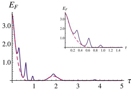
FIG. 7. (Color online)  $E_F$  for a Sub-Ohmic reservoir in the high- $T$  limit ( $k_B T / \hbar \omega_c = 100$ ) with  $\alpha = 0.1$ ,  $r = 2$ , and  $x = 0.3$ . The solid blue line is the exact solution while the dashed red line is the secular solution. The inset is a magnification of the temporal region  $0 \leq \tau \leq 1.5$ .
