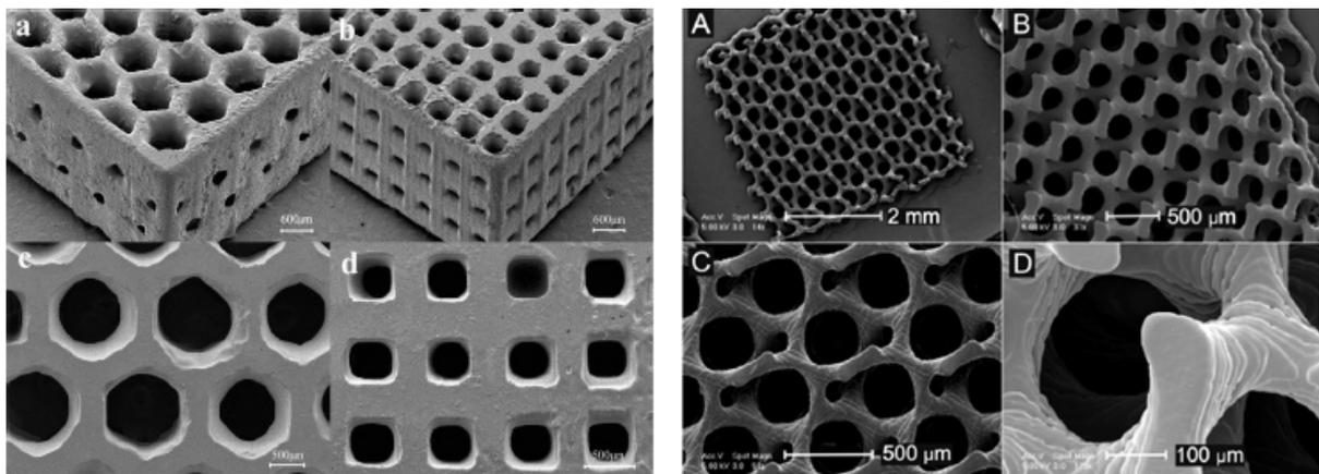
**Fig. 7.** Examples of tissue engineering scaffolds built by stereolithography using PPF or PDLLA-fumarate and a reactive diluent. Left: structures prepared from PPF and DEF as a reactive diluent [6]. Right: structures prepared from PDLLA-fumarate and NVP as a reactive diluent [5].
