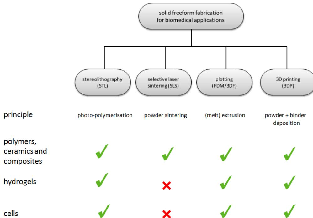
**Fig. 1.** Overview of additive processing/solid freeform fabrication technologies applied for biomedical applications. For each technique, the symbols indicate whether polymers and/or ceramics, hydrogels, and living cells have been employed.
