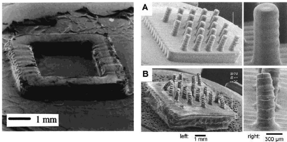
**Fig. 5.** SEM images of biodegradable structures built by stereolithography intended for application in tissue engineering. Left: structures prepared from P(TMC-co-CL)-coumarin macromers [9]. Right: structure prepared from P(TMC-co-CL)-acrylate (A) before and (B) after 1 month of implantation [8].
