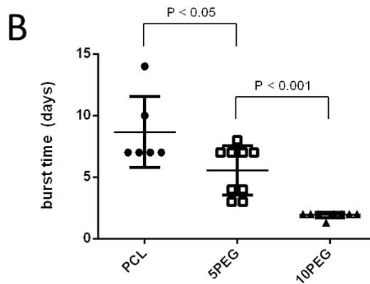
Figure 5. Osmosis-driven delayed burst release. A: relative weight increase of tubes filled with saturated glucose and dye for different polymer compositions upon immersion in PBS. B: delay times for release: mean, standard deviation and p-values (unpaired t-test, N=6-9).
