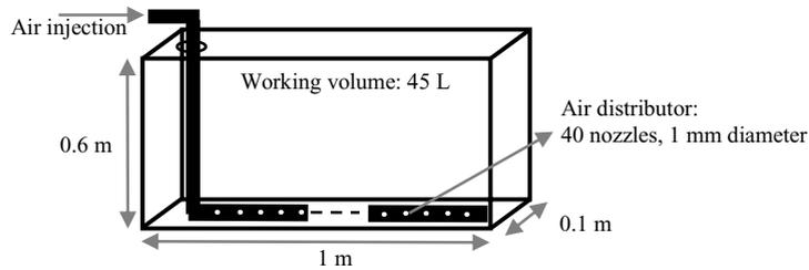
Fig. 1. The design of flat plate photobioreactor.
