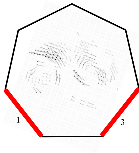
Fig. 5. Particle Velocity Imaging of the fluid when transducers 1-3 are excited simultaneously.
