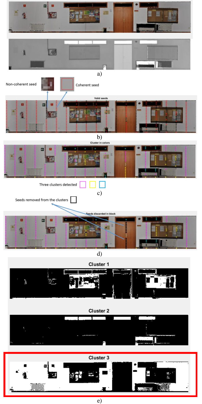
Figure 3. Wall's area detection. a) RGB image and depth image b) Searching valid small square patches (they are called seeds in the figure). c) Seed clusters. d) Removing inconsistent seeds from clusters. e) Segments and wall area identification (marked in red).
