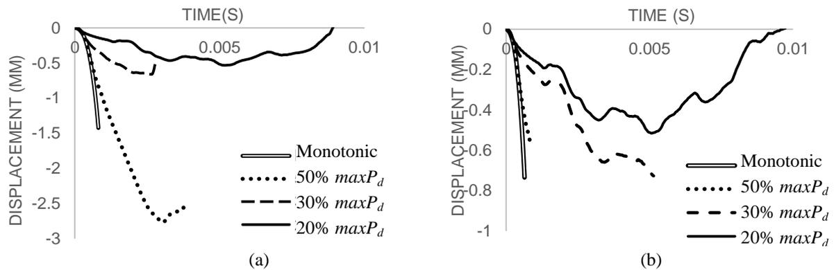
Figure 11 Predicted mid-span displacement time history obtained for pulse loads with  $\dot{P}=400\text{kN/ms}$  but different intensities for (a) Specimen C2 and (b) Specimen E1.
