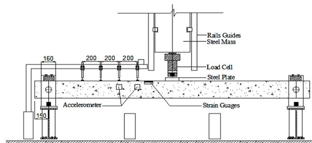
Figure 2 Drop-weight test setup employed at HWU
