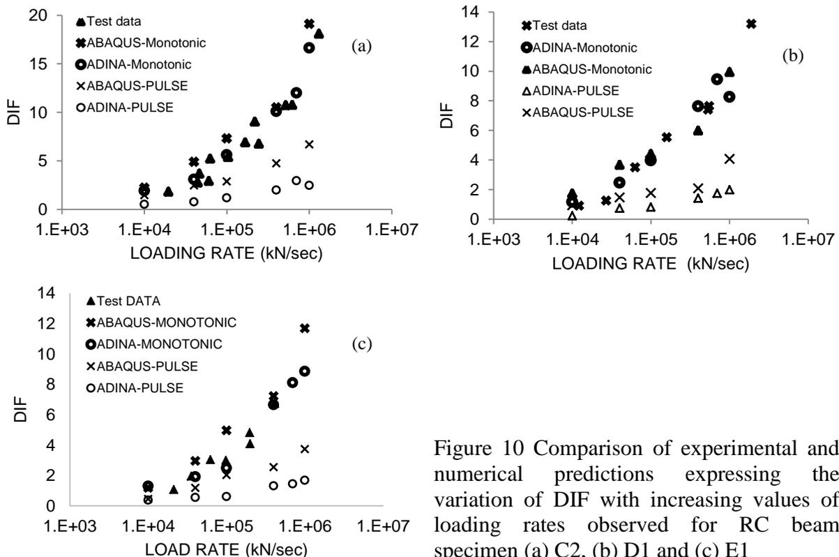
Figure 10 Comparison of experimental and numerical predictions expressing the variation of DIF with increasing values of loading rates observed for RC beam specimen (a) C2, (b) D1 and (c) E1
