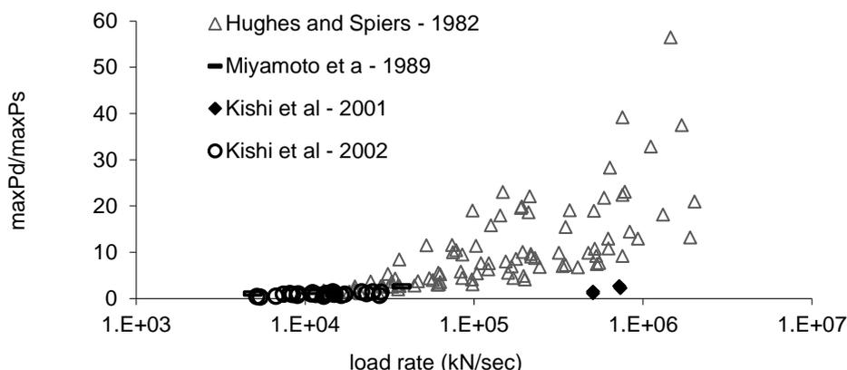
Figure 5 Variation of maximum sustained load during impact ( $maxP_d$ ) normalised by the static load-carrying capacity ( $maxP_s$ ) with increasing values of loading rate
