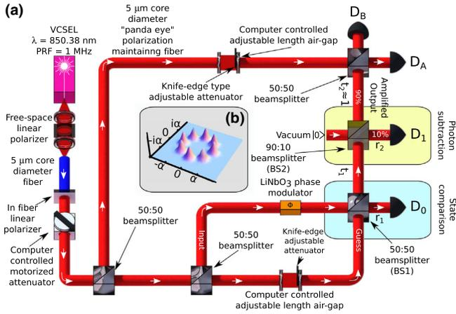
FIG. 1 (color online). (a) Experimental implementation of the quantum optical state comparison amplifier and output state analyzer. The system comprises two interferometers. Each  $D$  denotes a silicon single-photon detector [30]; VCSEL denotes a vertical cavity surface emitting laser and PRF the pulse repetition frequency of the laser. (b) Eight possible input coherent states.
