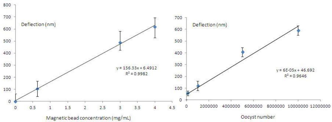
Figure 4. Plot of deflection (nm) against magnetic bead concentration (left graph) and oocyst number (right graph) showing a linear trends in cantilever response against magnetic bead concentration (confirming that the magnetic enhancement of detection is quantitative) and oocyst exposure.
