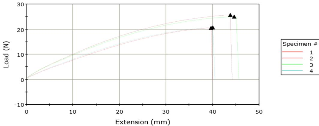
Figure 4 Load Vs Extension of PP fibre
