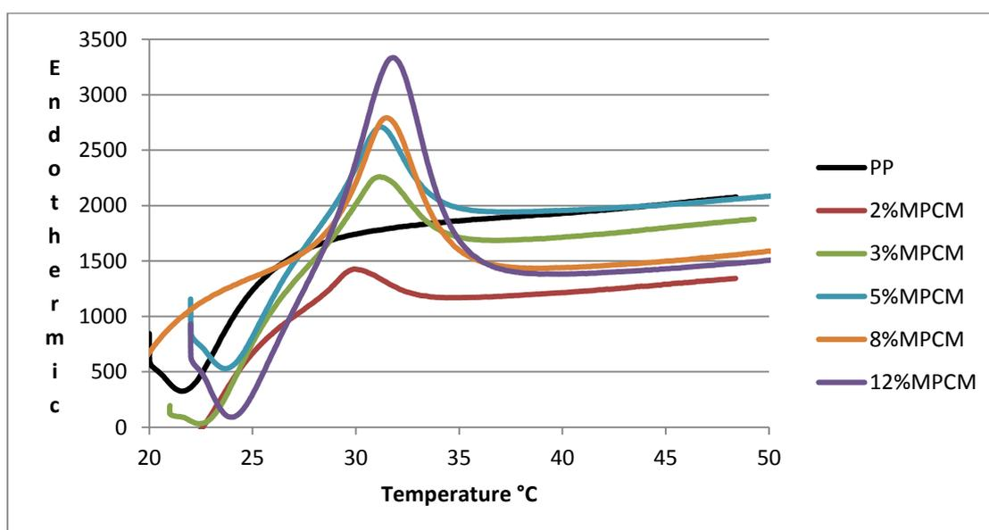
Figure 3 DSC graph showing latent heat of fibres with MPCM
