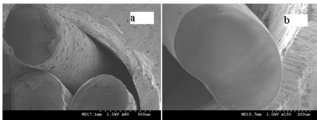
Figure 1 SEM images (a) with MPCM (b) without MPCM
